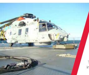
low-profile design and resultant under-fuselage clearance allows the handling of a wide range of helicopters and fixed wing aircraft in both land-based and marine operations. The unit will operate with aircraft that have deflated tires or collapsed oleos, and with nose installed radomes.
