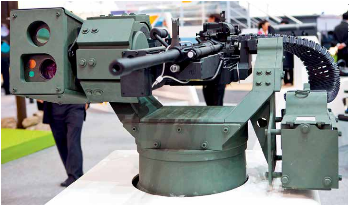
ST Engineering's ADDER is actually a family of RWS ranging from a lightweight single 7.62 machine gun mounting through dual. 50 MG/40mm AGL weapon configurations suitable for installation on wheeled or tracked vehicles.
