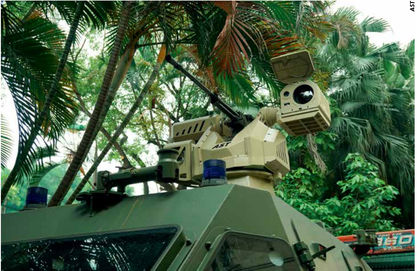
The ARROW-12 RWS was developed by AST of Singapore. It can accommodate 7.62mm, 12.7mm or 14.5mm machineguns in ground vehicle or naval applications. Various optic suites can be provided suitable for day and night engagement.
