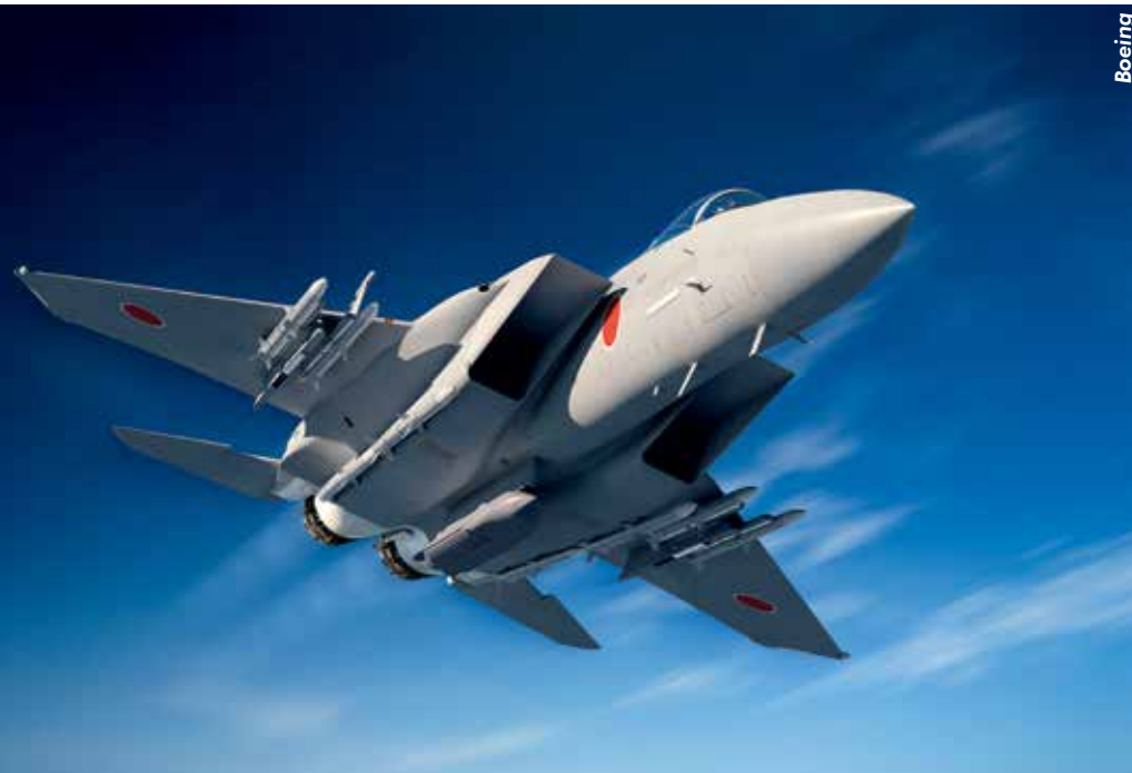
A rendering of an upgraded Japan Air Self-Defense Force F-15JSI loaded with air-to-air missiles and a single air-to-surface glide weapon on the centreline weapon pylon.
