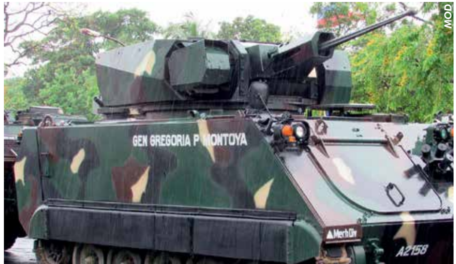
The Philippine Army upgrade of its M113 APC fleet by Elbit Defence includes both .50 and 25mm RWS. The relative straight forward modification illustrates one of the advantages provided by the RWS design.
