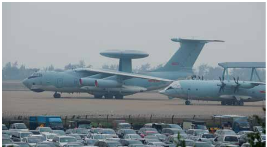
The KJ-2000 Y-8 'Moth' Balance Beam (foreground) and KJ-2000 (Mainring) airborne early warning and control (AEW&C) aircraft stand side by side.
