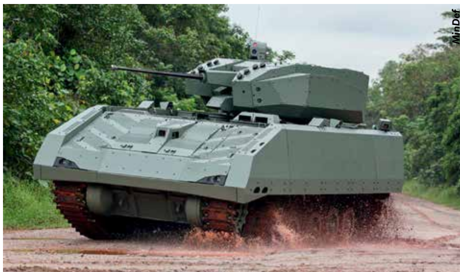
Singapore's Next Generation Fighting Vehicle – the Hunter – utilises an entirely unmanned weapon turret. The crew are positioned in the vehicle hull and use a suite of networked panoramic, perimeter, and sighting cameras for surveillance and target acquisition and engagement.
